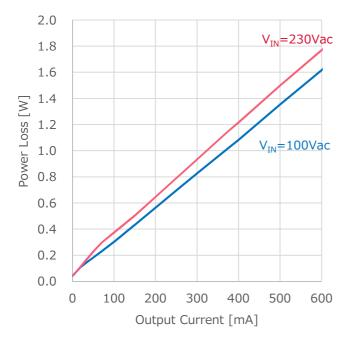
Figure 8. Load Regulation (I<sub>OUT</sub> vs. P<sub>LOSS</sub>)
