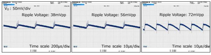
$V_{IN}$ =230Vac, IOUT=10mA Figure 18. VOUT Ripple Voltage.4
