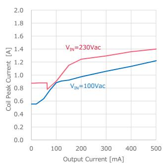
Figure 13. Coil Peak Current (I<sub>OUT</sub> vs. I<sub>peak</sub>)
