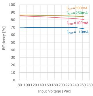
Figure 11. LINE Regulation (I<sub>OUT</sub> vs. Efficiency)
