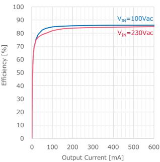
Figure 7. LOAD Regulation (I<sub>OUT</sub> vs. Efficiency)
