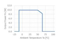
Figure 2. Temperature Deleting curve
