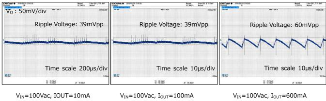
Figure 15. VOUT Ripple Voltage.1
