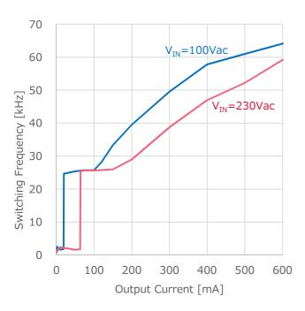
Figure 12. Switching Frequency (I<sub>OUT</sub> vs. F<sub>SW</sub>)
