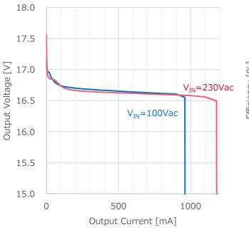
Figure 6. Load Regulation ( $I_{OUT}$  vs.  $V_{OUT}$ )
