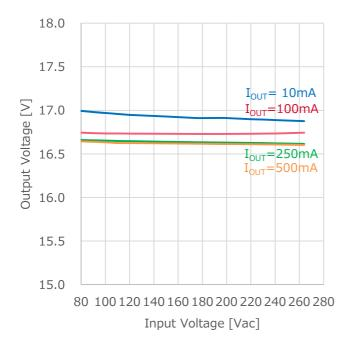
Figure 10. LINE Regulation ( $I_{OUT}$  vs.  $V_{OUT}$ )
