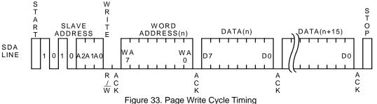
· With this command the data is programmed into the indicated word address.
