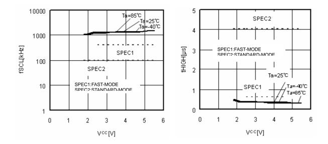
Figure 12. Clock Frequency fSCL
