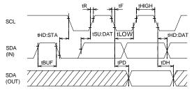
Figure 1-(a). Synchronous Data Timing
