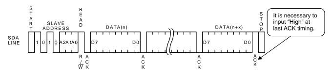
Figure 36. Sequential Read Cycle Timing (With Current Read)
