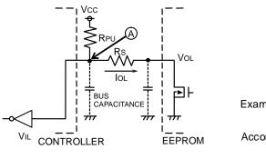
$$\frac{(V_{CC}-V_{OL})\times R_{S}}{R_{PU}+R_{S}} + V_{OL}+0.1V_{CC} \leq V_{IL}$$
