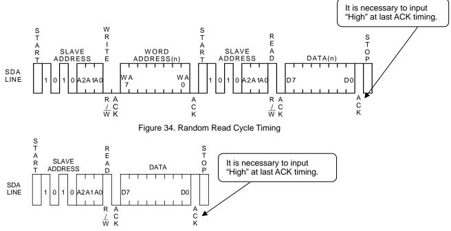
Figure 35. Current Read Cycle Timing
