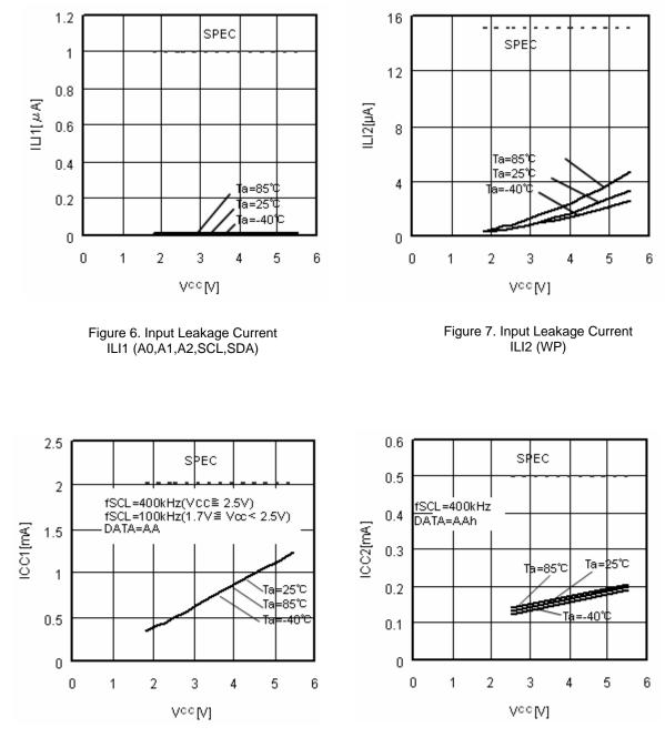
Figure 8. Write Operating Current ICC1 (fSCL=100kHz,400kHz)
