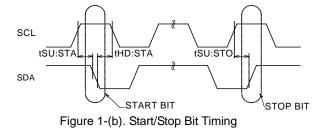
OSDA data is latched into the chip at the rising edge of SCL clock.
