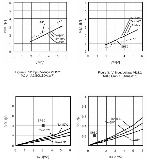
Figure 4. "L" Output Voltage VOL1-IOL1 (Vcc=2.5V)
