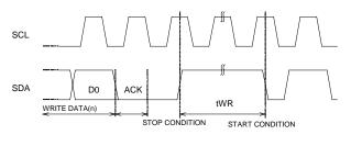
Figure 1-(c). Write Cycle Timing
