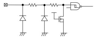
Figure 49. Input Pin Circuit
