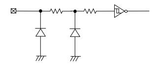
Figure 46. Input Pin Circuit
