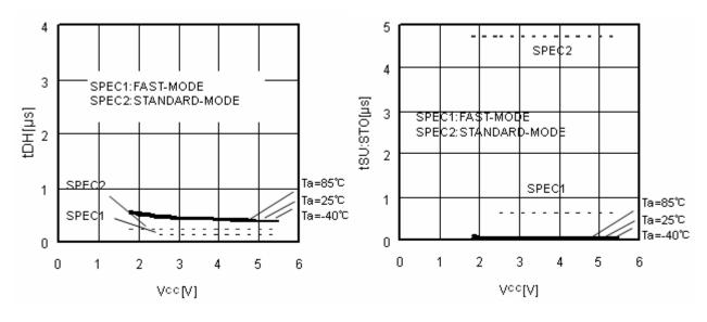
Figure 22. Output Data Hold Time tDH
