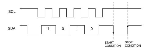
Figure 40. Command cancellation by the START and STOP conditions during input of the Slave Address
