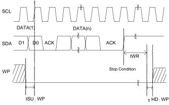
Figure 1-(d). WP Timing Of The Write Operation
