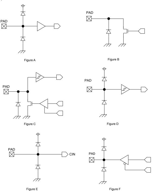
Figure BU21023GUL / BU21023MUV I/O Equivalent Circuit
