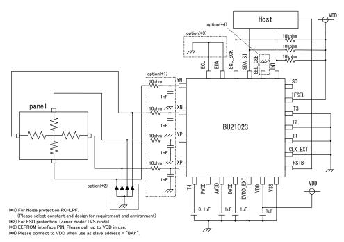
Example 2: BU21023GUL/MUV Application Circuit (2-wire Serial bus)
