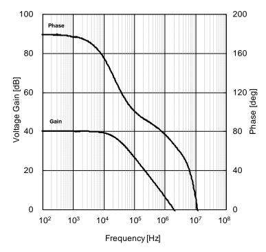
Figure 47. Voltage Gain · Phase vs Frequency
