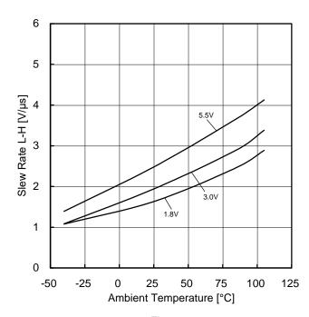
Figure 22. Slew Rate L-H vs Ambient Temperature
