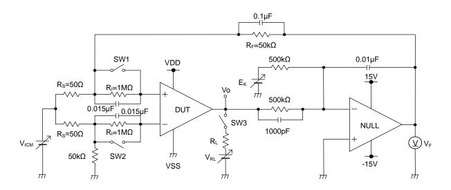
Figure 71. Test Circuit 1 (One Channel Only)
