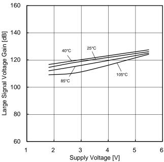
Figure 17. Large Signal Voltage Gain vs Supply Voltage
