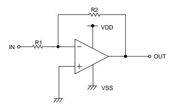
Figure 76. Inverting Amplifier Circuit
