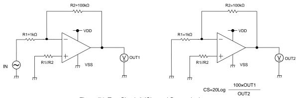
Figure 74. Test Circuit 3 (Channel Separation)
