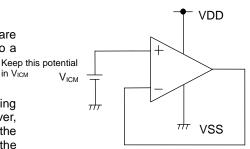
Figure 79. Example of Application Circuit for Unused Op-amp
