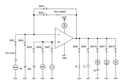
Figure 72. Test Circuit 2 (each channel)
