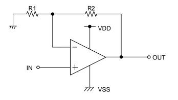
Figure 77. Non-inverting Amplifier Circuit
