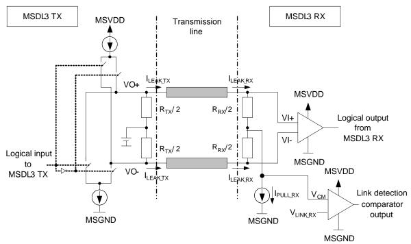
Fig.16. high-speed channel equivalent schematic.
