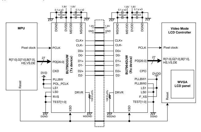
Fig.17. Application circuit
