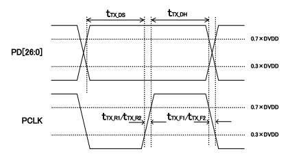
Fig.10 Parallel Data Input AC Timing
