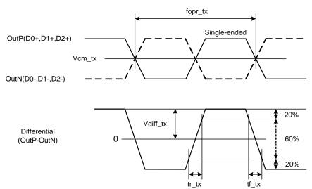
Fig.15. High-Speed Channel Electrical Characteristics
