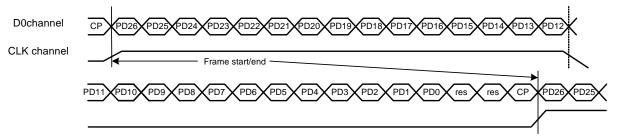
Fig.7. MSDL3 Protocol for 1-channel Data (27-bit)
