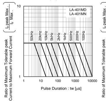
Fig.6 Ratio of Maximum Tolerable Peak Current vs. Pulse Duration ( III )
