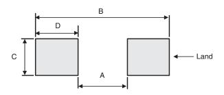
(Unit: mm) Dimensions С Type Code Α В D Part No. **MCR006** YZP 0.3 0.84 0.3 0.27 MZP MCR01 0.5 1.3 0.4 PZPI EZP MCR03 MZP 1.0 2.0 8.0 0.5 PZPI 2.6 MCR10 EZP 1.2 1.15 0.7 MCR18 EZP 2.2 4.0 1.5 0.9 MCR25 JZH 2.2 4.0 2.3 0.9 MCR50 JZH 6.0 2.3 3.8 1.1 MCR100 JZH 5.1 8.1 3.0 1.5
