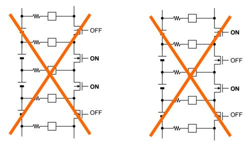
IC heats by cell balancing current and cell balancing switch resistor, restrict the number of switches of ON and time of ON, in order to keep the power consumption of cell balancing switch less than allowable power dissipation,
