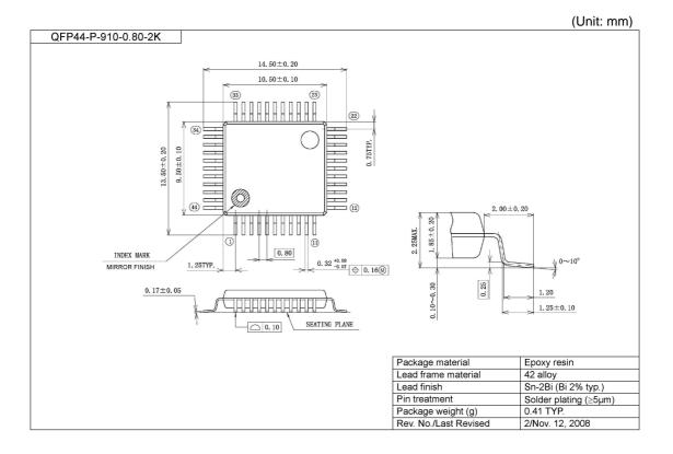
The surface mount type packages are very susceptible to heat in reflow mounting and humidity absorbed in storage. Therefore, before you perform reflow mounting, contact ROHM's responsible sales person for the product name, package name, pin number, package code and desired mounting conditions (reflow method, temperature and times).
