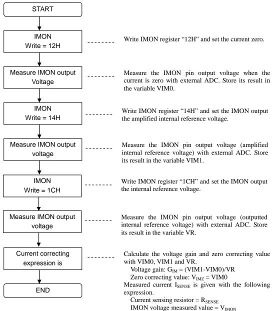
$I_{\text{SENSE}} = (V_{\text{IMON}} - V_{\text{IMZ}}) / G_{\text{IM}} / R_{\text{SENSE}}$
