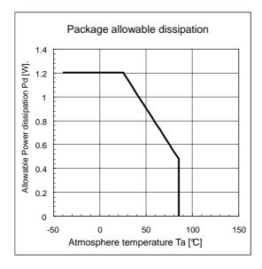
Package loss tolerant decreases as the atmosphere temperature (Ta) increase. If VREG pin output load current is large, make the power loss smaller than the value shown in this figure.
