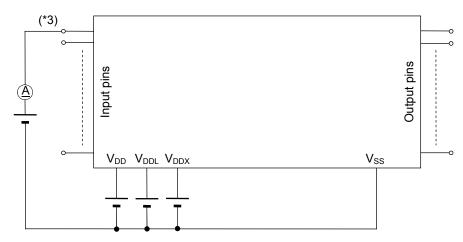
\*3: Measured at the specified output pins.
