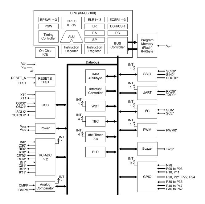
Figure 1 ML610Q482P Block Diagram
