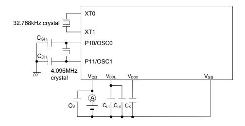
$\begin{array}{lll} \text{C}_{\text{V}:} & 1 \mu \text{F} \\ \text{C}_{\text{L}0:} & 1 \mu \text{F} \\ \text{C}_{\text{L}1:} & 0.1 \mu \text{F} \\ \text{C}_{\text{X}:} & 0.1 \mu \text{F} \\ \text{C}_{\text{GH}:} & 24 \text{pF} \\ \text{C}_{\text{DH}:} & 24 \text{pF} \\ 32.768 \text{kHz crystal:} \\ \text{C-001R (Epson Toyocom)} \\ 4.096 \text{MHz crystal:} \\ \text{HC49SFWB (Kyocera)} \end{array}$
