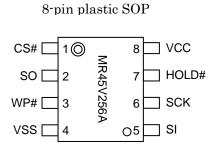
Note: Signal names that end with # indicate that the signals are negative-true logic.
