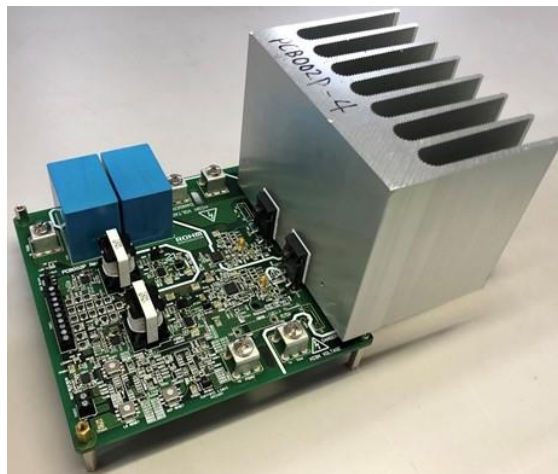
Figure 21. Heatsink Installation Example
