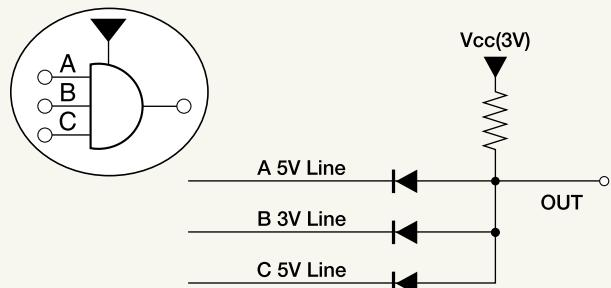
(Used when 5V signal line and 3V signal line co-exist.)
