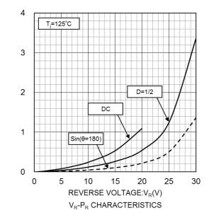
REVERSE POWER DISSIPATION:P<sub>R</sub>(W)
