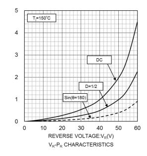
REVERSE POWER DISSIPATION:P<sub>R</sub>(W)
