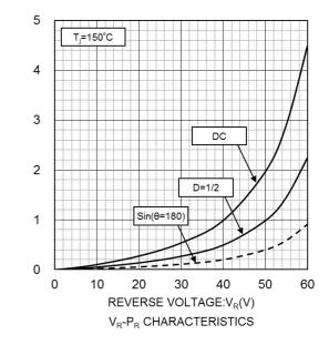
REVERSE POWER DISSIPATION:P<sub>R</sub>(W)
