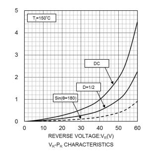
REVERSE POWER DISSIPATION:P<sub>R</sub>(W)
