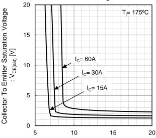
Gate To Emitter Voltage : V<sub>GE</sub> [V]
