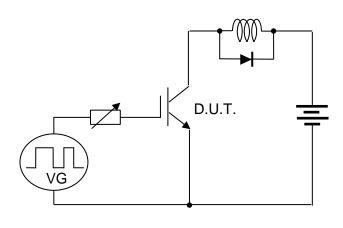
Fig.18 Inductive Load Circuit
