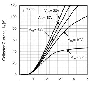
Collector To Emitter Voltage: V<sub>CE</sub>[V]
