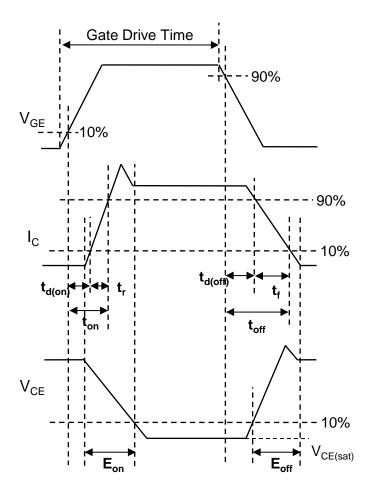
Fig.19 Inductive Load Waveform
