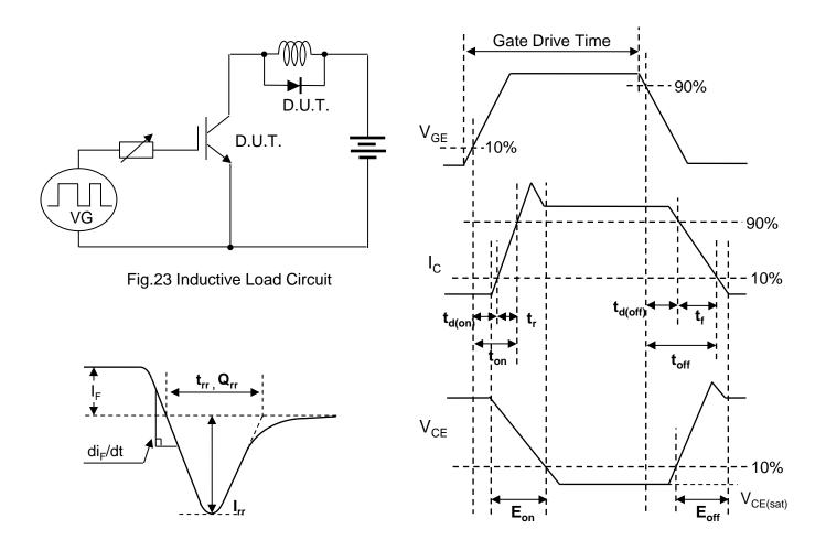
Fig.25 Diode Reverce Recovery Waveform
