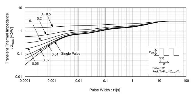
Fig.22 Diode Transient Thermal Impedance
