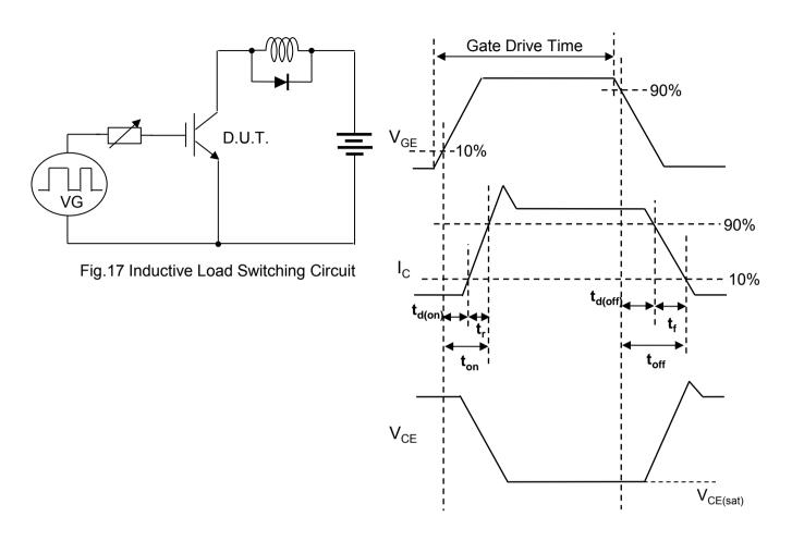
Fig.18 Inductive Load Switching Waveform
