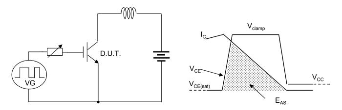
Fig.19 Self Clamped Inductive Switching Ciruit Fig.20 Self Clamped Inductive Switching Waveform
