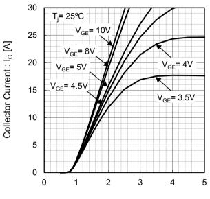
Collector To Emitter Voltage : V<sub>CE</sub>[V]
