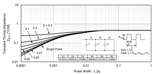
Fig.17 IGBT Transient Thermal Impedance
