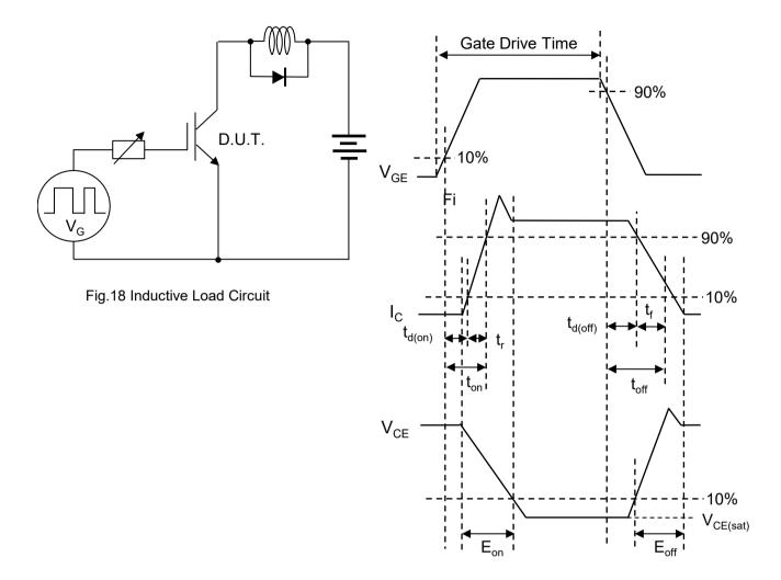
Fig.19 Inductive Load Waveform
