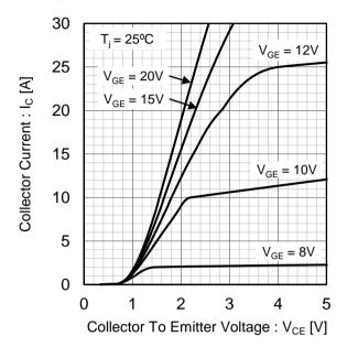
Fig.6 Typical Output Characteristics
