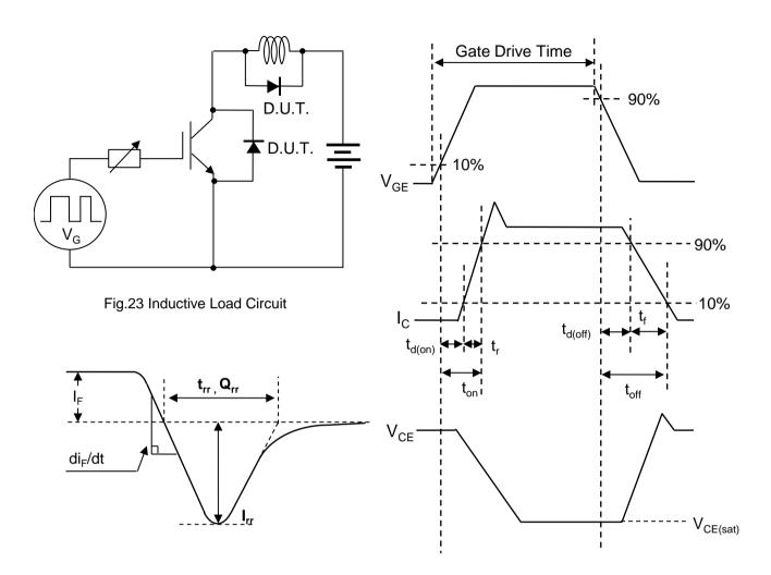
Fig.25 Diode Reverse Recovery Waveform
