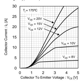
Fig.7 Typical Transfer Characteristics
