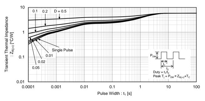
Fig.22 Diode Transient Thermal Impedance
