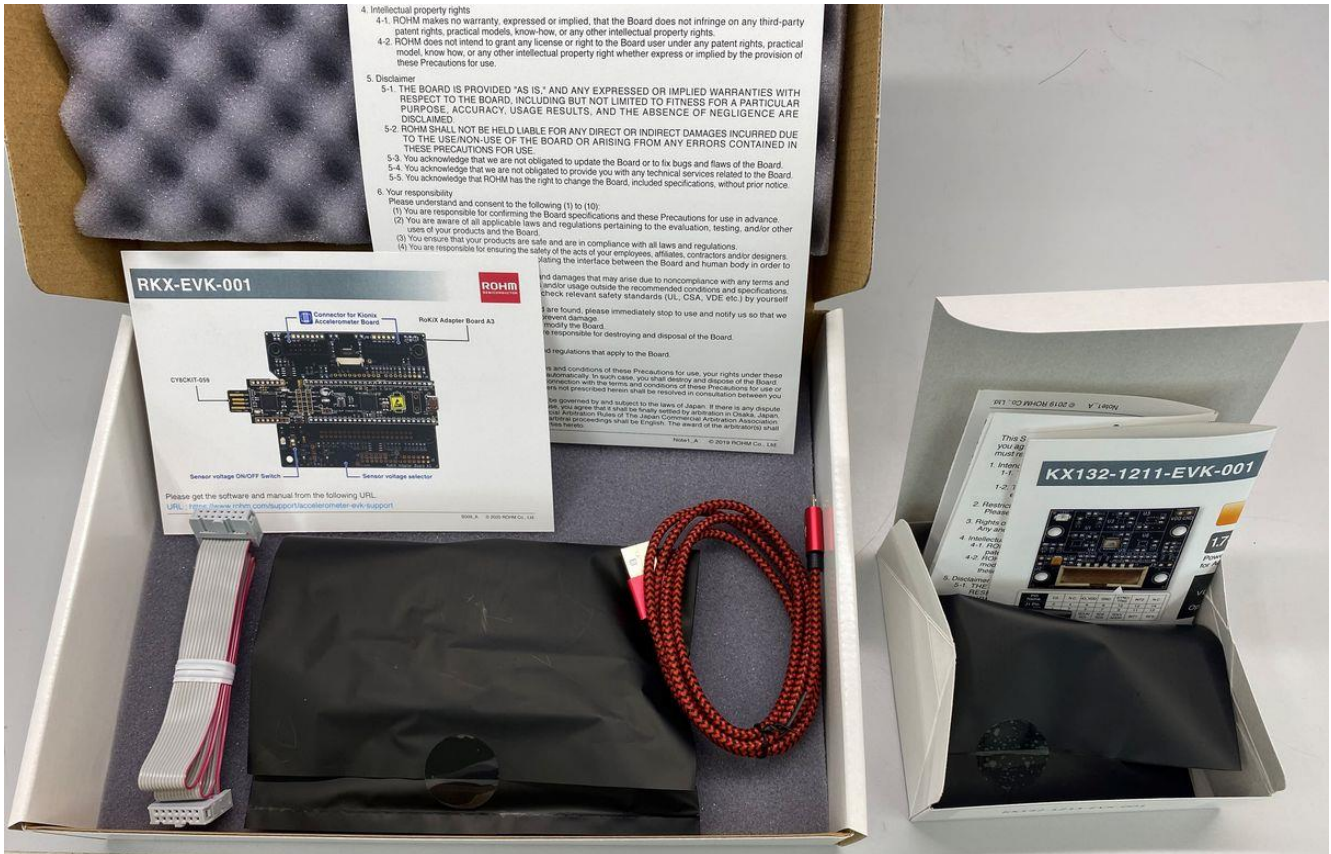
Figure 1. RKX-EVK-001 (Left) and RoKiX Digital Evaluation Board purchased separately (Right) shown here together
