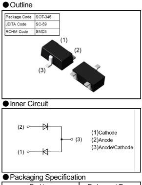
**Embossed** Tape Packing Reel Size(mm) 180 Taping Width(mm) 8 3000 Quantity(pcs) Taping Code T146 D5M Marking
