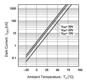
Fig.10 Output Characteristics
