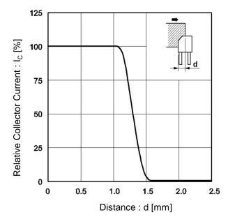
Fig.2 Relative Output Current vs.Distance (II)
