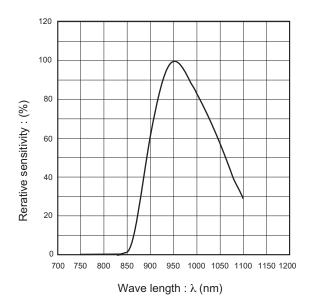
Fig.8 Optical bandwidth of the photo-diode encapsulation
