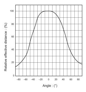
Fig.9 Direction characteristic (Horizontal direction)
