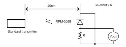
Fig.2 Measurement of standard transmitter proofreading
