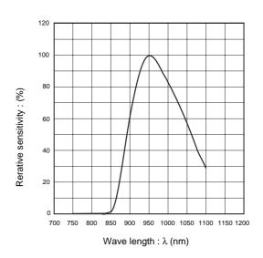
Fig.7 Optical bandwidth of the photo-diode encapsulation
