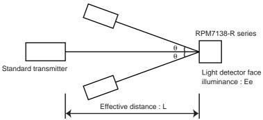
Fig.3 Measurement condition for effective distance
