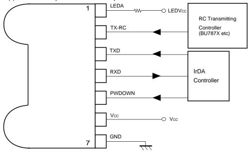
$<sup>\</sup>cdot \square$  of TX-RC (2pin) and TXD (3pin) in the table above is supposed to be the pulse input.
