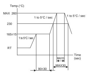
Condition of partial heat method (by soldering iron) is used;
