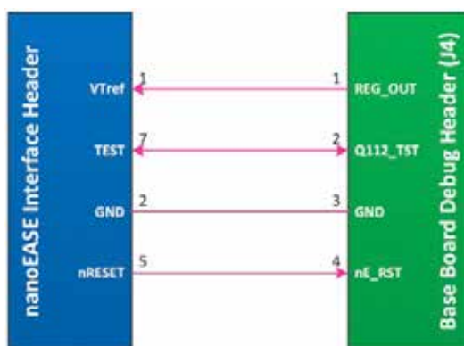
Figure 38: nanoEASE - Base Board Connection Diagram
