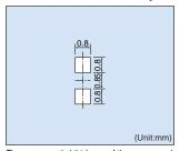
The recommended thickness of the screen mask for soldering is between 100 and 150 $\mu m$ . The hole size of the screen mask should be same as the recommended land pattern or smaller.
