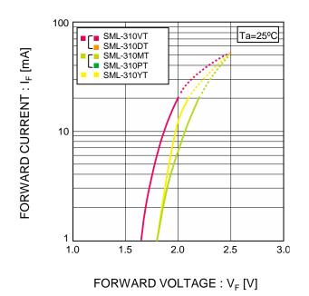
Fig.1 Forward Current - Forward Voltages
