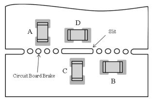
Stress strength according to the mounting position: A>B>C>D
