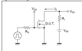
Fig.2-1 Gate Charge Measurement Circuit
