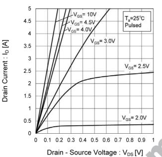
Fig.6 Typical Output Characteristics(II)
