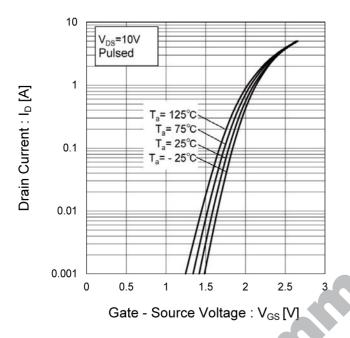
Fig.9 Gate Threshold Voltage vs.
