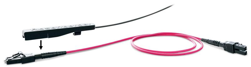
2) Switch the IDP light source on, light spot occurs at the rear wall of the connector body at the far end
