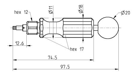
All dimensions are in mm; tolerances according to ISO 2768 m-H
