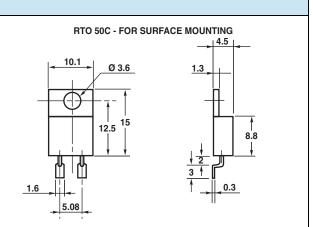
• Only for RTO 50 version C = during surface mount soldering, the soldering temperature profile must not cause the metal tab of this device to exceed 220 °C.
