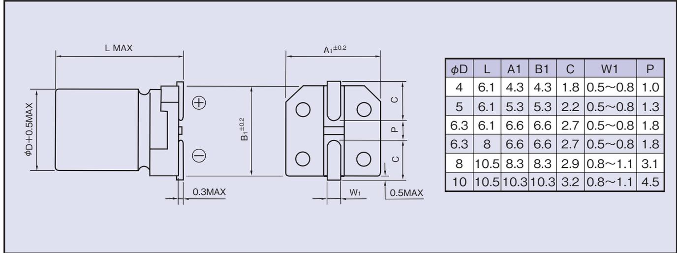
◆标准品一览表 / STANDARD SIZE Size φD×L(mm), Rated Ripple Current (mA r.m.s./105°C, 100kHz), Impedance(Ω MAX/20°C, 100kHz)
