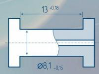
5000 turns, wire Ø0,063 mm coil resistance 870
