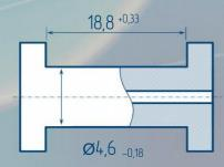
5000 turns, wire Ø0,063 mm coil resistance 550
