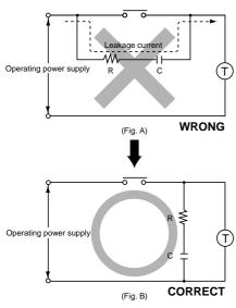
When a contact switch having an operation indicating lamp (lamp equipped limit switch, etc.) is used to apply power to the timer, a resistor having a value equal to or greater than the value below shall be connected in series with the lamp.
