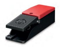
Analog Output Operation -As the pedal is depress, voltage or amperage (depending on model) is increase. Features an additional programmable NP NO signaling contact that activates at a preset level.
