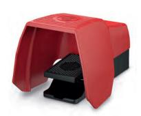
Standard OFF-ON Operation -Push pedal to change contact state. Release pedal to return to original state. Two Stage Operation-Press Pedal to change the state of the first set of contacts. Continue to press further to change the second set of contacts. Latching Operation Push pedal to change contact
