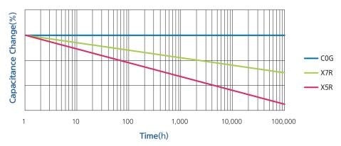
[ Example of Capacitance Aging ] \* Sample : COG, X7R, X5R
