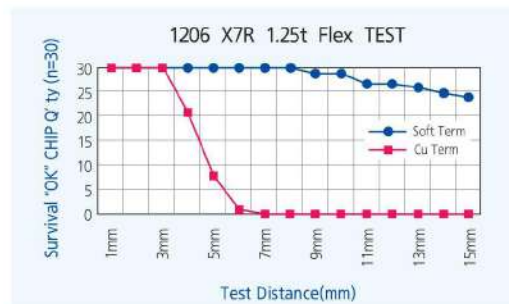
Soft - Termination relaxes the applied thermal - mechanical stresses by ductile properties of metal - polymer composites.
