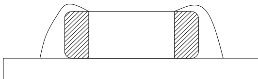
Too Much Solder large stress may cause cracks
