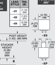
End Shroud (-075 post height only. Mates only with CLP.) (5.46 mm) .215" to (15.49 mm) .610"
