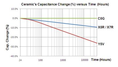
The capacitance value can be restored (a.k.a. 'de-aged') by exposing the component to elevated temperatures approaching its Curie Temperature (approximately 120°C). This 'deaging' can occur during the component's solder-assembly onto the PCB, during life or temperature cycle testing., or by ' baking ' at 150°C for about 1 hour.
