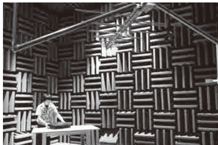
Acoustic radio wave anechoic chamber
