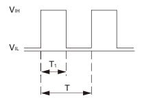
$V_{IH}=4.75$  to 5.25 V  $V_{IL}=0$  to 0.4 V PWM duty cycle (%) =  $\frac{T_1}{T} \times 100$  PWM frequency 25 (kHz) =  $\frac{1}{T}$  Current source (Isource) = 1.0 mA max. (when control voltage is 0 V) Current sink (Isink) = 10 mA max. (when control voltage is 5.25 V)
