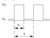
$V_{IH} = 2.8 \text{ to } 5.25 \text{ V}$   $V_{IL} = 0 \text{ to } 0.4 \text{ V}$ PWM duty cycle (%) =  $\frac{T_1}{T} \times 100$ PWM frequency 25 (kHz) = Current source (Isource) = 2 mA max. (when control voltage is 0 V) Current sink (Isink) = 2 mA max. (when control voltage is 5.25 V) Control terminal voltage = 5.25 V max. (when control terminal is open)
