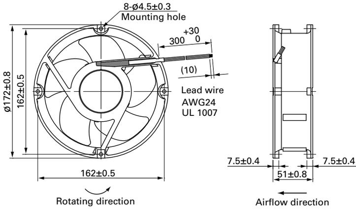
**Reference Dimensions of Mounting Holes and Vent Opening (unit: mm)**
